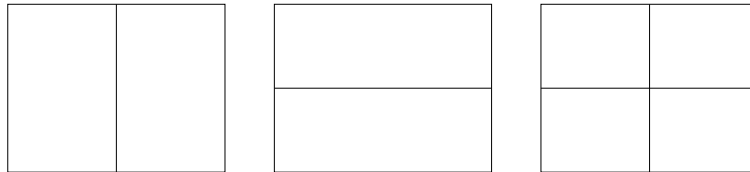
Figure 2.2: Refinements in 2d, from left to right: refinement in direction e_1 , e_2 , and both
